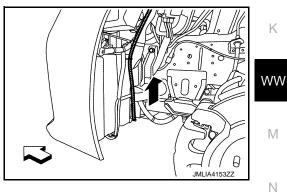
3. Remove washer tube from portion (A) of washer tank, and then pull out washer tube from clips (B).
