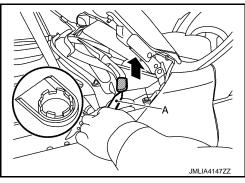
3. Remove wiper arm fixing nut, and then remove wiper arm.
