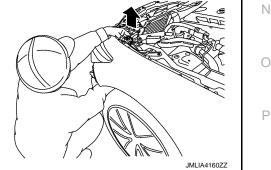
b. Remove washer tank inlet.
