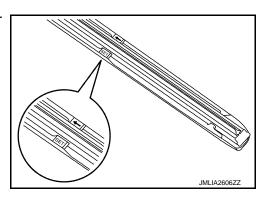
2. Pass through pawl of wiper blade in the groove of wiper refill. **NOTE:**
