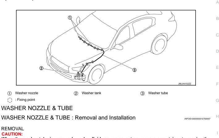
When the washer tube is removed, washer fluid may come out so prepare a container to receive the fluid and never allow fluid to be sprinkled.
